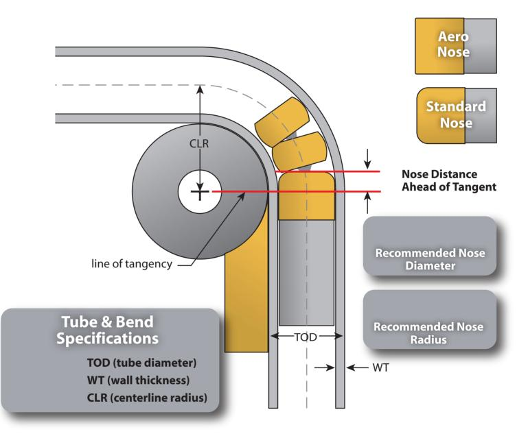
Note: this set-up utility is designed to provide a starting point for proper set-up. Mandrel may require adjustment forward or backward of this recommendation based on other set-up variables.
